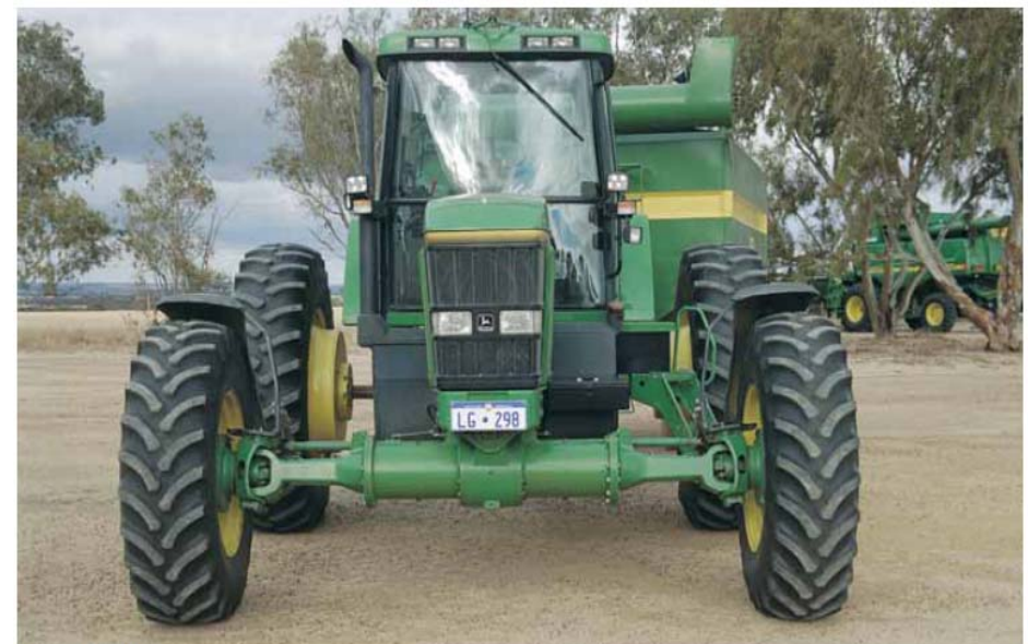
Photo 7.2 This John Deere tractor has had the front axle extended to 3 m centres
