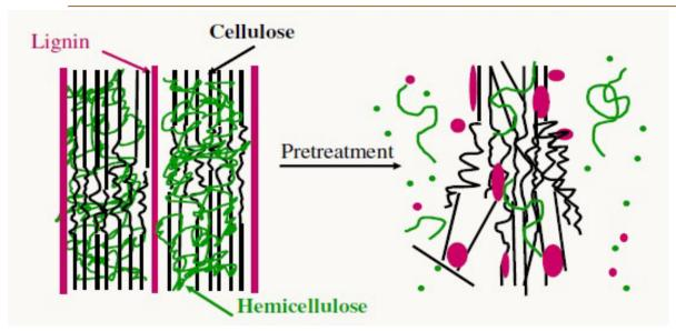
Steam at high pressure T: 150-210°C 5-10 min Acid catalyst
